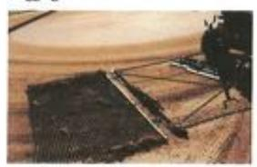
To perform this task, a mat drag is the most affordable and effective tool available. It can be pulled by hand or by a piece of equipment. A standard size mat drag, 72" wide by 40" long, is most effective when field conditions are dry. When field conditions are wet, a standard size mat drag that has been folded or a mat drag that has been shortened to 12" to 18" long should be used.
